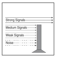
If the gate is set just right (SQUELCH set properly), just the desired signals get through.
